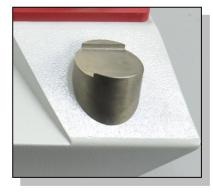
Install abrasion test sample, can put fixture here to make it closer.
