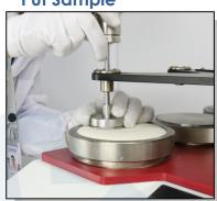
After put sample for abrasion test, put weights according to standards.
